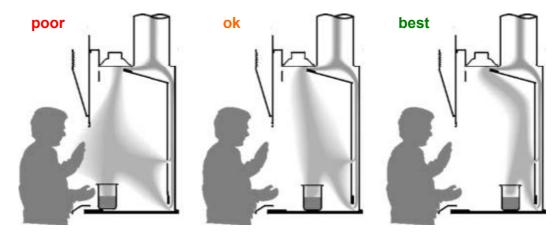
(I) If it is absolutely necessary to store material or instruments in the cupboard, a shelf or legs should be used to raise the obstruction by at least 5 cm to allow airflow underneath to the baffle opening:
