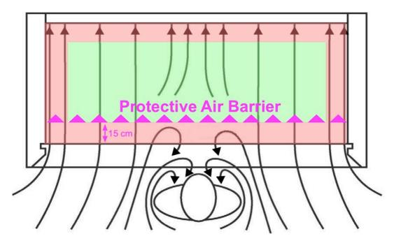
(k) Most of the air entering a fume cupboard travels across the work surface and behind the baffle at the back. Do NOT block the back baffle opening just above the base. Optimum protection is offered approximately 15 cm in front of the baffle:
